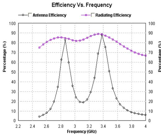
**Fig. 5.** Radiation & antenna efficiency graph
